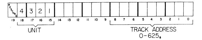
Bits 0 - 8 specify the track to be loaded. This is an octal number between 0 and 625. Loading a higher numbered track will result in the disk not being able to acknowledge successful execution of this command. Only bits 0 - 8 are loaded. Tracks 0 - 17 are reserved for use by DEMON and reading or writing on these tracks will result in its complete exorcism.
