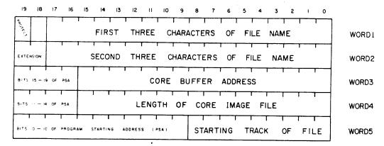
Bit 19 is set if a file is protected. Bits 18 and 19 of WORD 2 constitute the extension. A binary number from 0-3 can be expressed in these bits. On a directory listing a letter will be printed for each number.
