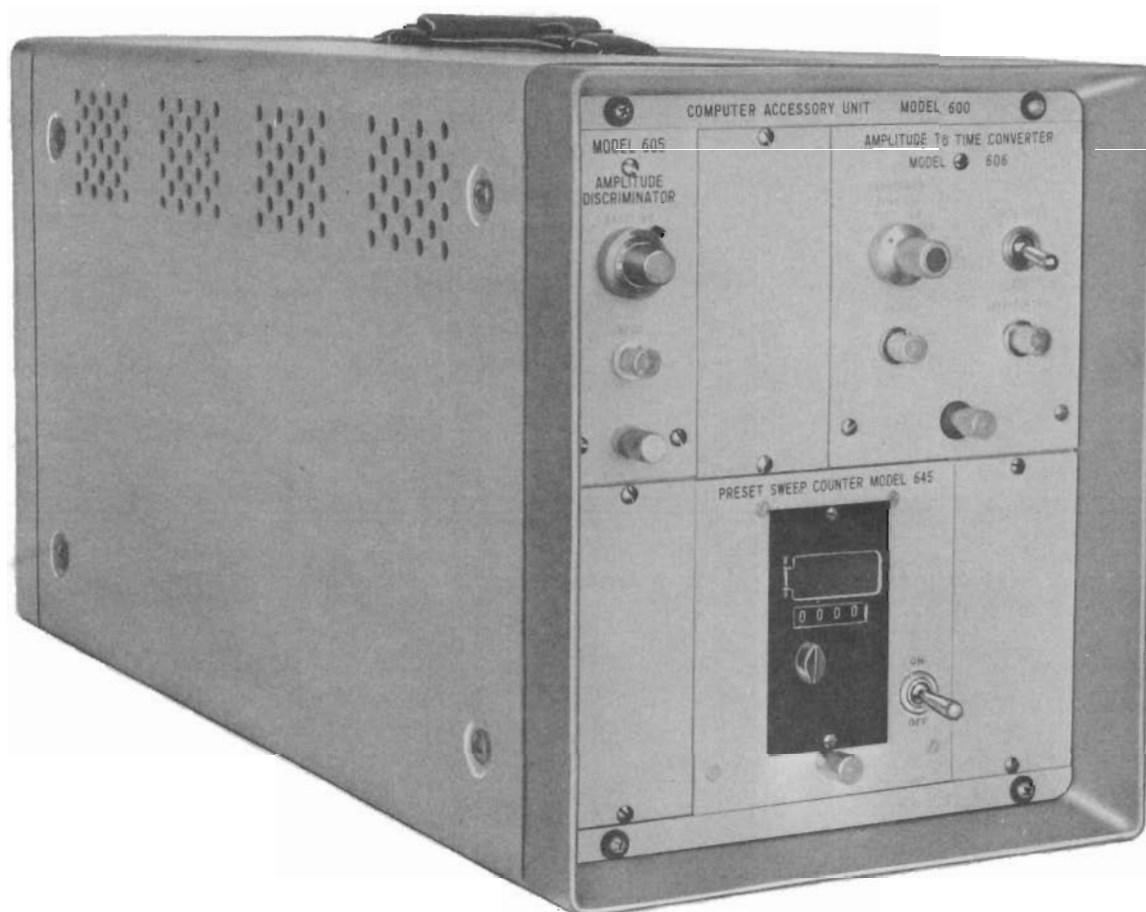
Figure 1-1. Series 600 CAT Accessory Cabinet showing Model 605 Amplitude Discriminator, Model 606 Amplitude-to-Time Converter, and Model 645 Preset Sweep Counter.
